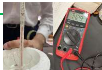
Sample of data collection of the resistance of a thermistor sensor using a multimeter and a thermometer.
